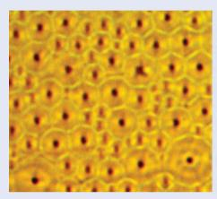
of cholesteric liquid-crystal oligomers. A polygonal array (see left panel of image) forms during the annealing step; this structure is then frozen by the quenching step.
