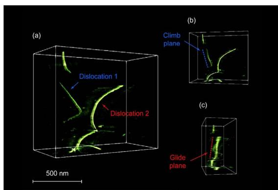
*Elucidation of deformation mechanisms in TiAl at 900°C, thanks to 360° 3D vision. (a) Volume of nanometric dimensions containing two dislocation loops. (b-c) Visualization of the volume from different angles, allowing to identify crystallographic planes of climb and glide for these two dislocations.*
