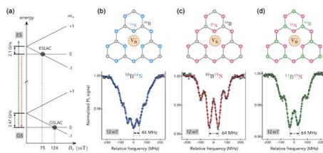
(a) Simplified energy level structure of the  $V_B^-$  center in hBN showing the electron spin sublevels  $m_s = 0, \pm 1$  in the ground (GS) and excited states (ES), as well as their evolution with a static magnetic field  $B_z$  applied along the  $c$ -axis of hBN. Hyperfine structure of the  $V_B^-$  center in (b) h  $^{10}\text{B}$   $^{14}\text{N}$ , (c) h  $^{10}\text{B}$   $^{15}\text{N}$ , and (d) h  $^{11}\text{B}$   $^{15}\text{N}$  crystals.
