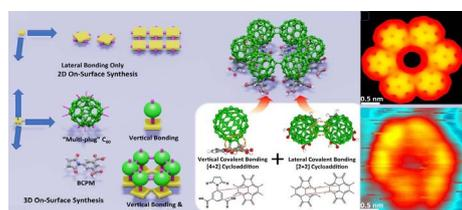
Figure 1. Schematic diagram of 3D synthesis-on-surface. On right, the STM images of the obtained "six-petal flowers" of covalently coupled C<sub>60</sub> (bottom : experimental, top: calculated image) bonded on the top of six self-assembled BCPM
