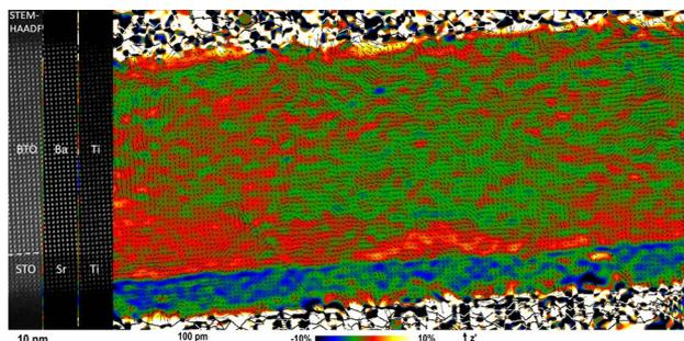
Decomposition of cross-sectional HR-STEM-HAADF image of  $\text{BaTiO}_3$  (BTO)-on- $\text{SrTiO}_3$  (STO) structure into images of sub-structures of Ba + Sr atoms and Ti atoms. Background: map of out-of-plane strain  $\epsilon_{zz}^{\text{BTO}}$  of Ba+Sr sub-structure with reference to BTO Bravais lattice obtained by AbStrain. Arrows: relative displacement between the sub-structure of Ti atoms and the sub-structure of barycenters of Sr or Ba atoms obtained by Relative displacement
