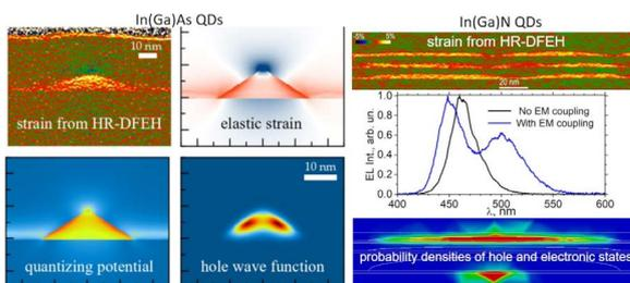
Two dimensional out-of-plane strain maps obtained by dark-field electron holography in high-resolution mode in In(Ga)As (on the left) and In(Ga)N (on the right) QDs used for 3D strain and composition fields reconstruction within finite element and  $\vec{k} \cdot \vec{p}$  calculations and the modeled optoelectronic properties of such QDs.
