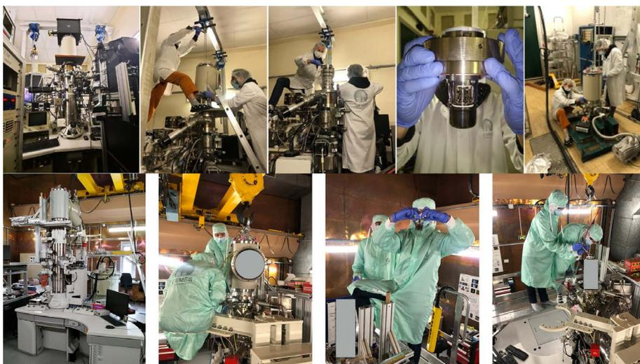
Figure 1: Pictures of the gun transfer from femtoTEM to HC-IUMI. Top: removal of the ultrafast gun assembly from FemtoTEM. Bottom: Installation in HC-IUMI by S. Meuret and H. Lourenço-Martins.
