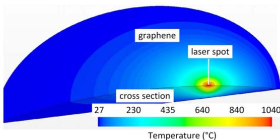
Temperature distribution of graphene bubble when heated with a laser spot obtained by numerical finite volume analysis.
