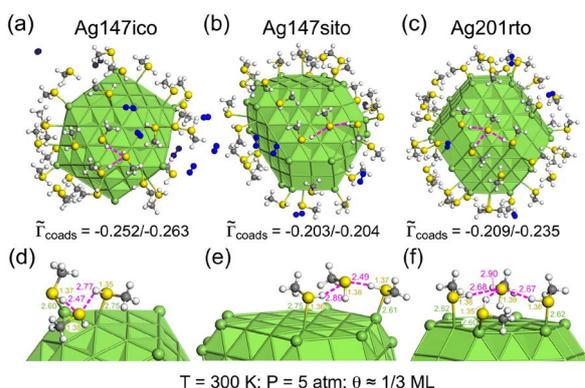
Illustration of final structures for contaminated Ag NPs immersed in gaseous nitrogen (5 atm), equilibrated at 300 K, extracted from AIMD trajectories and optimized in accurate conditions of (a) Ag147ico, (b) Ag147sito and (c) Ag201rto. In each case, an example of a coadsorption species composed of three or four methanethiol molecules is extracted from the optimized structures and depicted below them (d) Ag147ico (e) Ag147sito and (f) Ag201rto.
