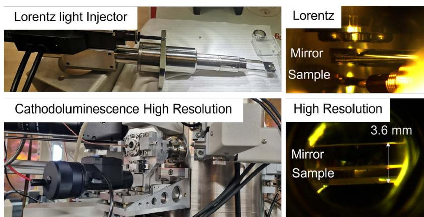
Figure 2: The two light injectors designed and built by the mechanical department. Top: the Lorentz injector with the flat mirror, left outside the column and right a view of the mirror and the sample in the microscope chamber. Bottom: High resolution injector with the system attached to the column (left) and the visualization of the HR chamber with a pole piece gap of 3.6 mm (right).
