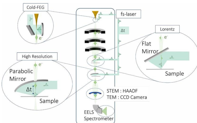
Figure 3: Sketch of the HC-IUMI microscope with the laser driven cold-field emission gun and the two samples position (Lorentz and high resolution).
